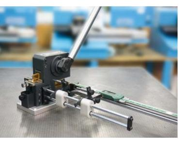
An indispensable handheld device. 3 devices in one. Multifunctional and with digital gauge. The mcut|multi can not only cut rules, but also lips. And it can also notch. For rule materials from 2 pt to 3 pt. It cuts steel quickly and without deformation. And it does so with a very small footprint.
