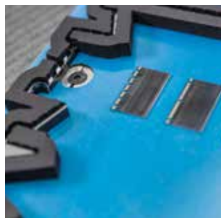
Rule pieces with various nick configurations.
