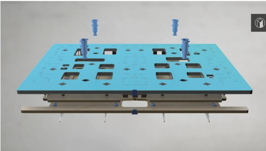
Insider tip for cigarette box production: the masterstrip|plate is also available with pre-breaking of flaps. For flaps that open perfectly. And a trouble-free packing process.
